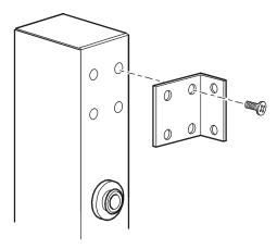
2. Attach the PDU to a vertical-mounting rail in the rear of the enclosure using two additional screws per bracket (not provided).
